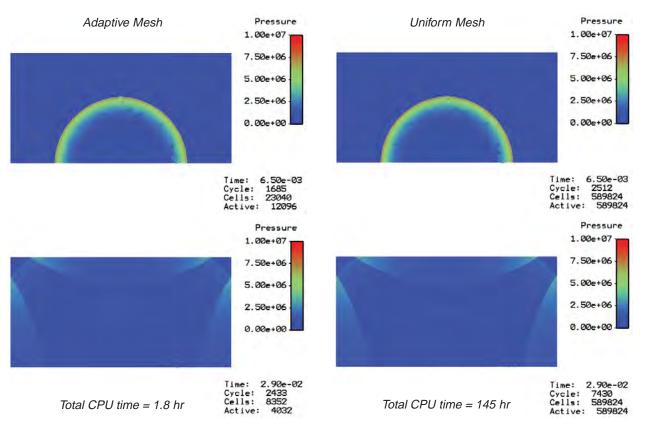
Figure 1. Comparison of adaptive mesh refinement (left) and uniform mesh solutions (right) for a 2-D blast wave computation in CTH. AMR, finite element error analysis, and mesh partitioning algorithms are being used to improve the efficiency of existing CSM analysis tools such as CTH and EPIC.
