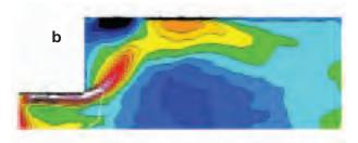
Figures 1a and b. Isocontours of axial velocity in the combustor for two different swirl numbers (left S = 0.56, right S = 1.12). The colors red and green indicate left-to-right flow, whereas blue and black indicate reverse flow. As shown, increase in swirl creates a recirculating (reverse flow) bubble in the combustor that pushes the flame outward and also stabilizes the combustion.
