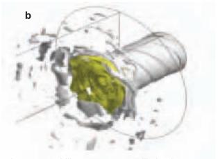
Figures 2a and b. Increase in swirl (left to right) in a premixed system stabilizes pressure oscillation in a gas turbine and also directly impacts the flame (yellow)-vortex (gray) interaction process. With high swirl, the shear layer at the dump plane breaks down, and a recirculation bubble forms in the combustor that stabilizes the flame; hence the combustion process.
