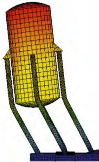
d. 3-D finite-element grid with 3-D load
