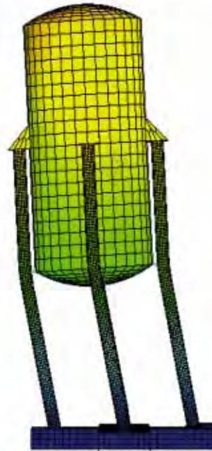
b. 3-D finite-element grid with experimental load
