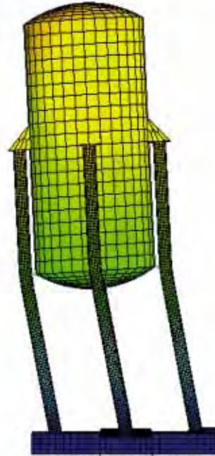
b. 3-D finite-element grid with experimental load
